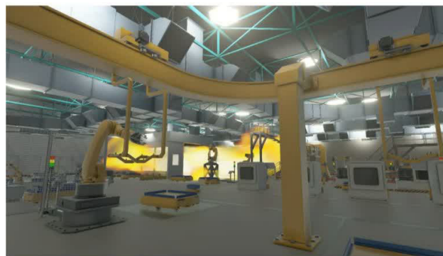
Figure 3. A vapour cloud explosion in a confined space using realistic geometry modelled in the CFD modelling software FLACS.
