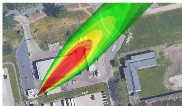
Figure 2. A high-pressure release of hydrogen, simulated using the integral modelling software EFFECTS.
